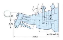
WARNER Hydraulic Vee-Drive. A Warner gear coupled to a Walter vee-drive. Ratios of 1.29:1, 1:67:1, and 2:1. Weight 135 lbs. Turns left hand propeller. WARNER Hydraulic Gear. In-line construction with no offset. Available with direct drive and 1½, 2, 2½ and 3 to 1 ratios for left hand propellers, and 1.9:1 for right hand propellers. Weight, direct drive 96 pounds, reduction gear 147 pounds.
