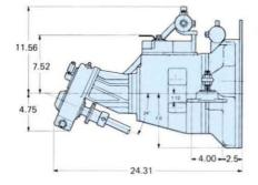
PARAGON Hydraulic Vee-Drive. A Paragon P20 hydraulic gear close-coupled to a Walter vee-drive. Ratios of 1.29:1, 1.67:1, and 2:1. Weight 132 lb. Turns left hand propeller. SAO Paragon direct manual gear. Weight 58 lb. Turns left hand propeller. Also shown, reduction gear with 1½:1 and 2:1 ratios. Weight 82 lb. Turns left hand propeller.
