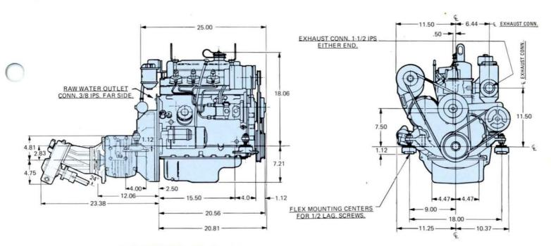
WESTERBEKE Short Profile Sailing Gear. The most compact 2:1 reduction package ever! Features positive neutral for free-wheeling, silent-running shaved case-hardened helical gears, heavy-duty tapered roller bearings, and instant acting fingertip control. (Use Morse 33C cable or equal.) Weight 25 lbs. Turns right hand propeller. Drawing above shows Walter vee-drive close coupled to the sailing gear. Reduction, 2:1. Weight 70 lbs. Turns right hand propellor.
