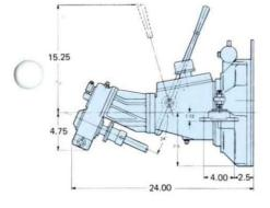
PARAGON SAOV. Use our front end exhaust outlet with this manual vee-drive. Available in ratios of 1.29:1, 1.67:1 and 2:1. Weight 90 Ib. Turns left hand propeller. PARAGON P20 Hydraulic Gear. Available with direct drive and in 1½, 2, 2½ and 3 to 1 ratios. The small offset (see table) can be turned down or up to suit the installation. Weight, direct drive 100 pounds, reduction gear 150 pounds. Turns left hand propeller.
